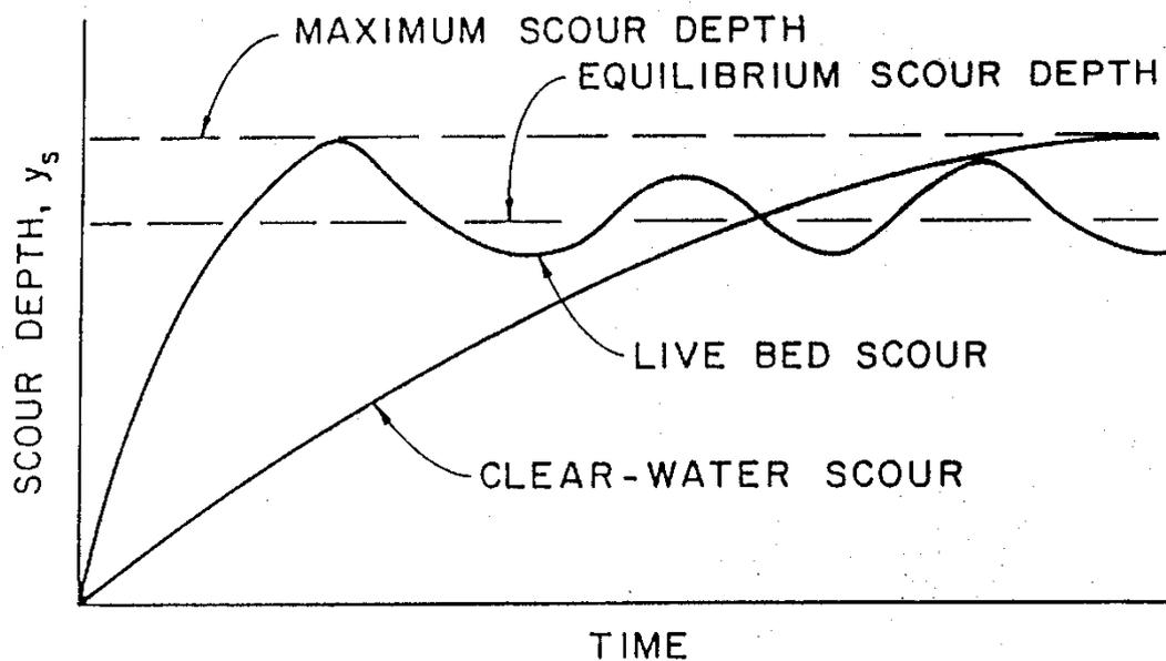
Figure 5.1 Live Bed Scour and Clear Water Scour as a Function of Time
