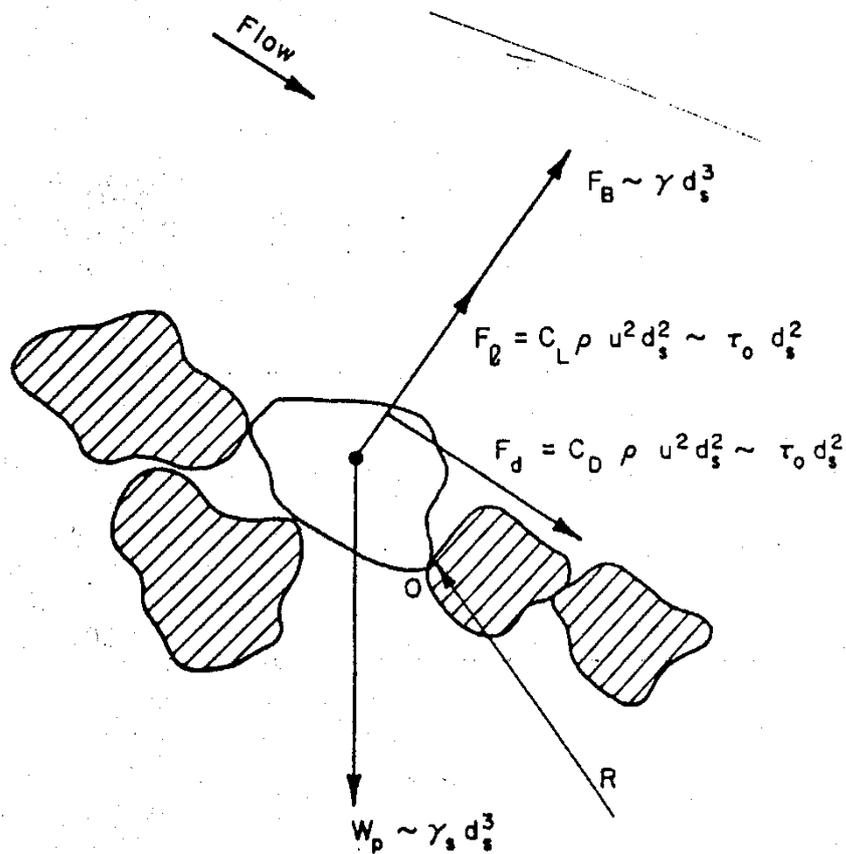
**Figure 3.1** Forces Acting on a Particle
