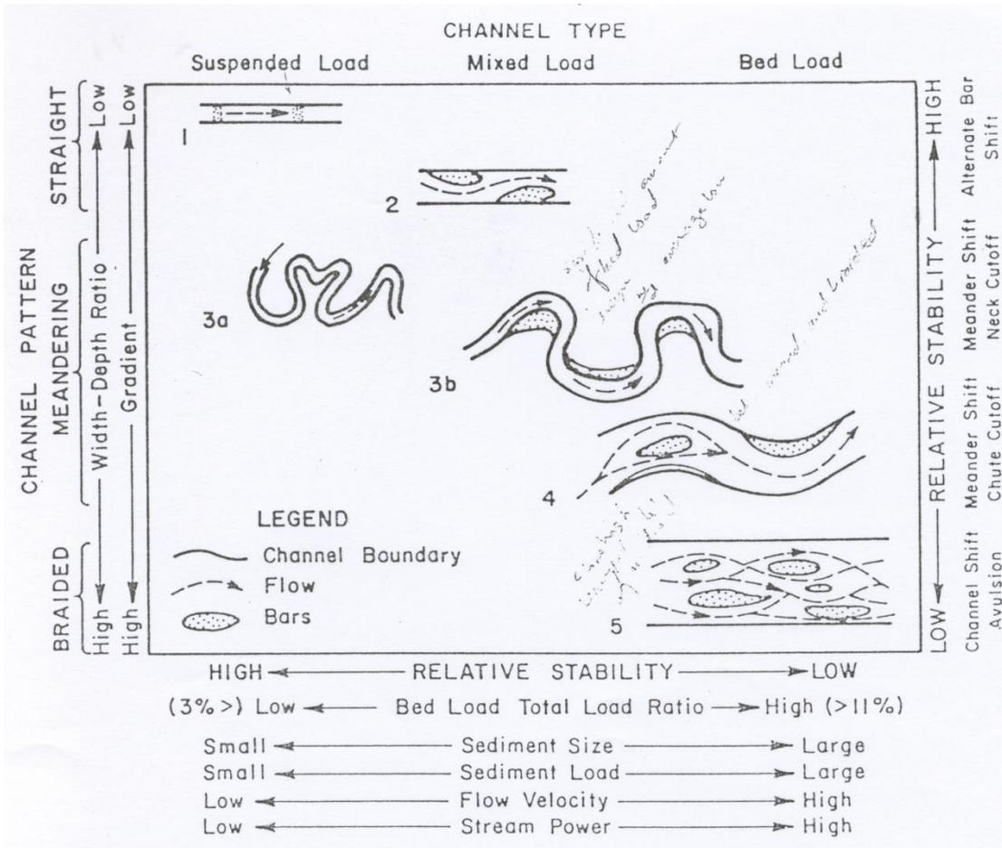
**Figure 7.1 Channel Classification After Shen et al. 1981**
