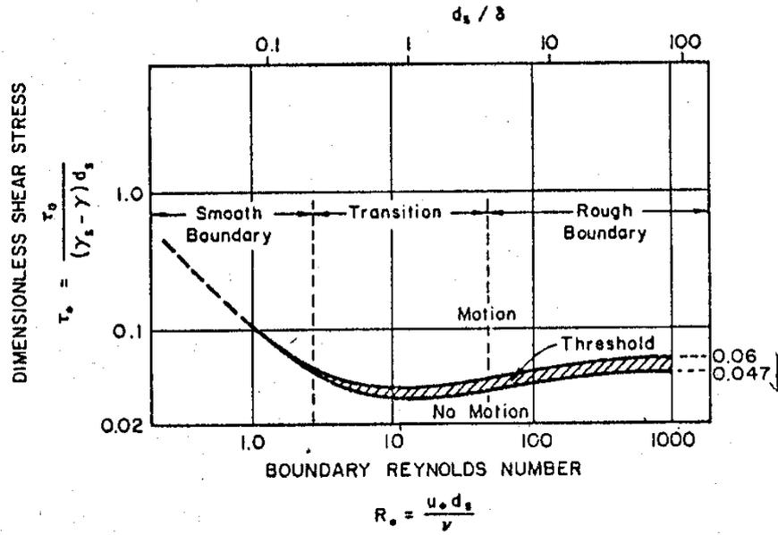
**Figure 3.2 Shields Diagram**
